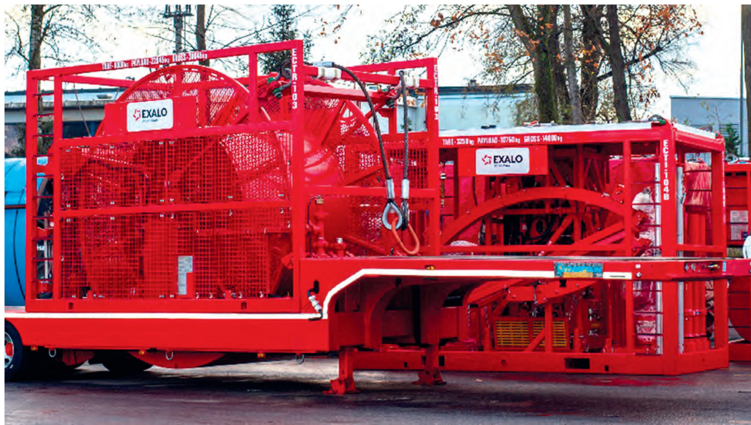
Fot. 6. Jednostka Coiled Tubing Hydra Rig. Arch. Exalo Drilling S.A.
